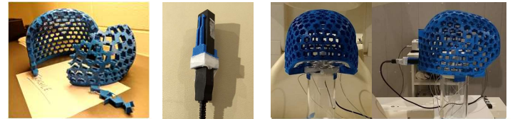
(a) Helmet (b) Sensor Jacket (c) Example of Experimental Setup Figure 3. 3D printed components
